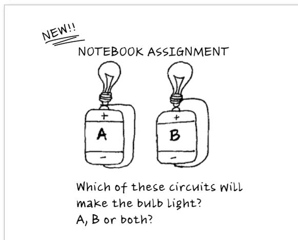
Although children constructed these very circuits, most students incorrectly predict that both bulbs will light. (The bulb in Circuit A does not.)
